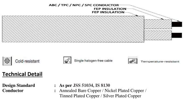
**Conductor Size** : Variant as per customer specifications **Conductor Type** : Solid wire / Flexible No of Core : Single Core / Multi Core **Core Insulation** : Extruded FEP Insulated **Core Formation** : Twisted **Inner Sheath Insulation** : Extruded FEP Insulated **Core Colour** : As per Customer specification. **Outer Sheath Colour** : As per Customer specification. Cable Temp. Range : Up to 200 Deg C **Voltage Grade** : Upto 1100 V
